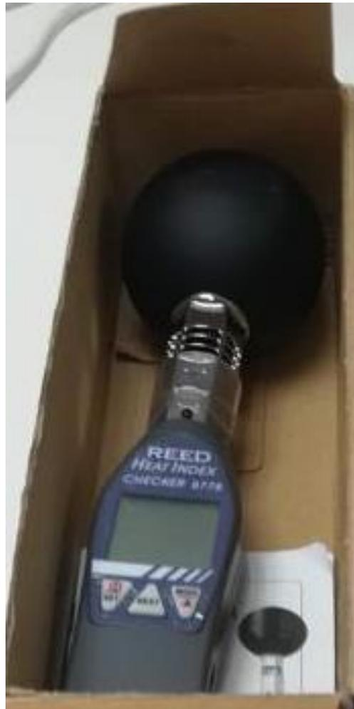
**Figura No. 7:** WBGT REED Heat Stress Meter Model 8778
