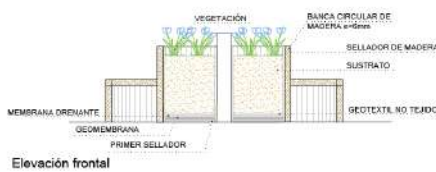
DETALLE 04: BANCA CIRCULAR
